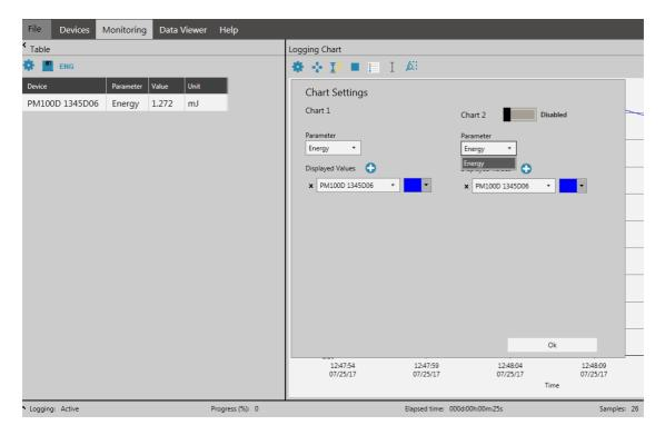
The **Logging Chart** displays the pulse energy values in a continuous line. Please adjust the saving interval according to the interval between the laser pulses in your setup to avoid data point without signal. For pulse intervals shorter than the saving interval, the displayed value is the last value sent by the power meter. For higher resolution measurements, please use the **Scope** mode.
