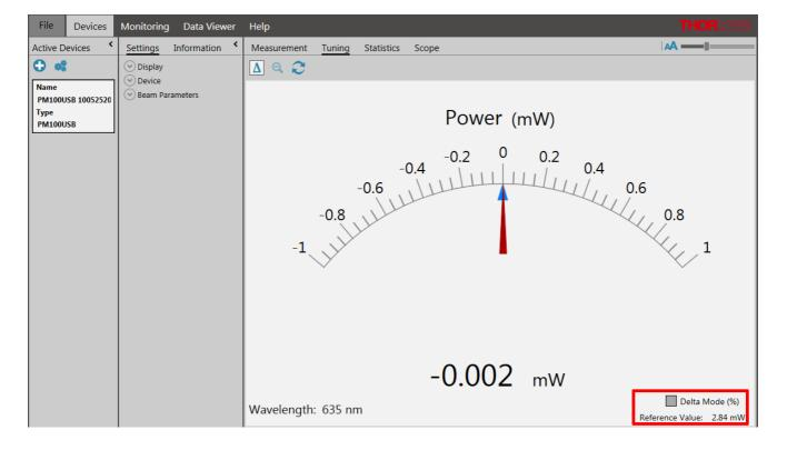
View the **Delta Mode** in % by selecting the tick-box: **Delta Mode (%)** in the lower right display, marked red.
