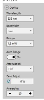
**Wavelength:** Set the wavelength of the measured light. This is essential in order to compensate the measurement result for the wavelength-dependent responsivity of the sensor.
