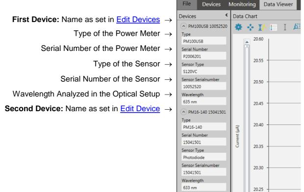
Go to the **Data Chart** and use the **Tool Bar** to configure the display of devices and parameters.
