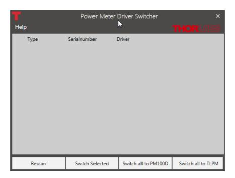
Use the **Menu Bar** at the bottom, to **Rescan** and see all attached devices. The table lists the **Type** of instrument, its **Serial Number** and the currently installed **Driver**.
