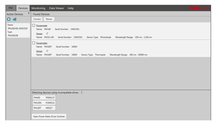
This is because the Thorlabs Optical Power Monitor uses a different driver for the connected power meters than former Thorlabs Power Meter software applications. For information on which driver to choose, click i for information or read the section Instrument Driver for Thorlabs Power Meters in this manual.
