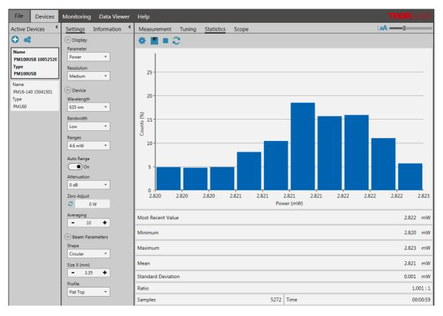
The chart displays the distribution of counts in percent for the parameter selected in <u>Settings</u>. This parameter can be changed during the active measurement. When parameter or monitored device are changed, the OPM starts a new data acquisition for statistical analysis.
