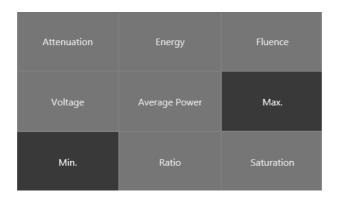
**Average Power:** The Average Power is calculated as an average of 3 measurement values. The calculation of the measurement values is based on the set **Averaging**.
