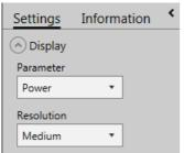
**Parameter:** Select the parameter that should be displayed as the main parameter in all 4 measurement monitors: Measurement, Tuning, Statistics and Scope.
