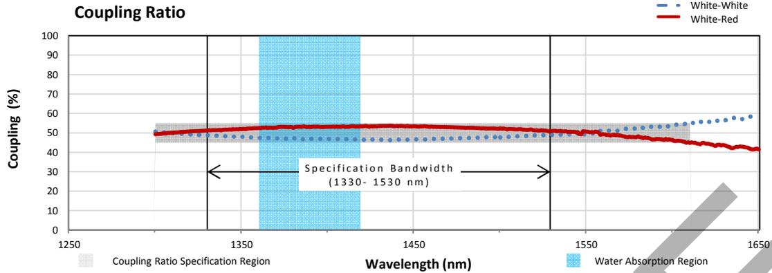
Coupling ratio (%) is the ratio of the optical power from each output port to the sum of the total power of both output ports as a function of wavelength. It is not impacted by the water absorption region because both output legs are affected equally.
