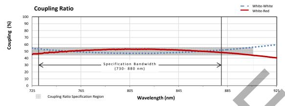
Coupling ratio (%) is the ratio of the optical power from each output port to the sum of the total power of both output ports as a function of wavelength.
