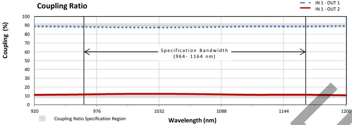
Coupling ratio (%) is the ratio of the optical power from each output port to the sum of the total power of both output ports as a function of wavelength.
