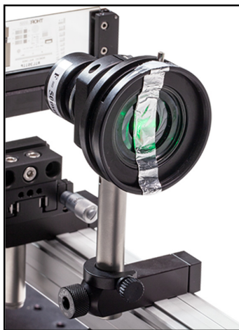
Figure 2: Aluminum foil strip blocking center of the aperture stop.
