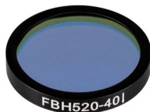
Figure 4: Bandpass filter (we use this as an excitation filter). The light should go through the filter in the direction of the arrow (note arrow on right in the label, right after the “-40”).
