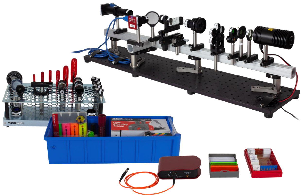
Figure 1 Overview of the optical microscopy setup. The kit contains an open rail with all optical components to go through the teaching steps. Furthermore, the kit contains a research grade spectrometer, various samples and tools to experiment, learn and evaluate.
