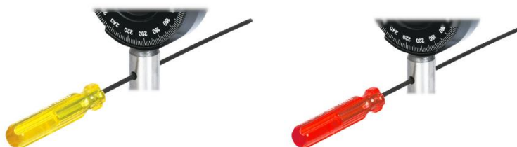
Figure 6 Using the balldriver for leverage on a Ø1/2" Post.
