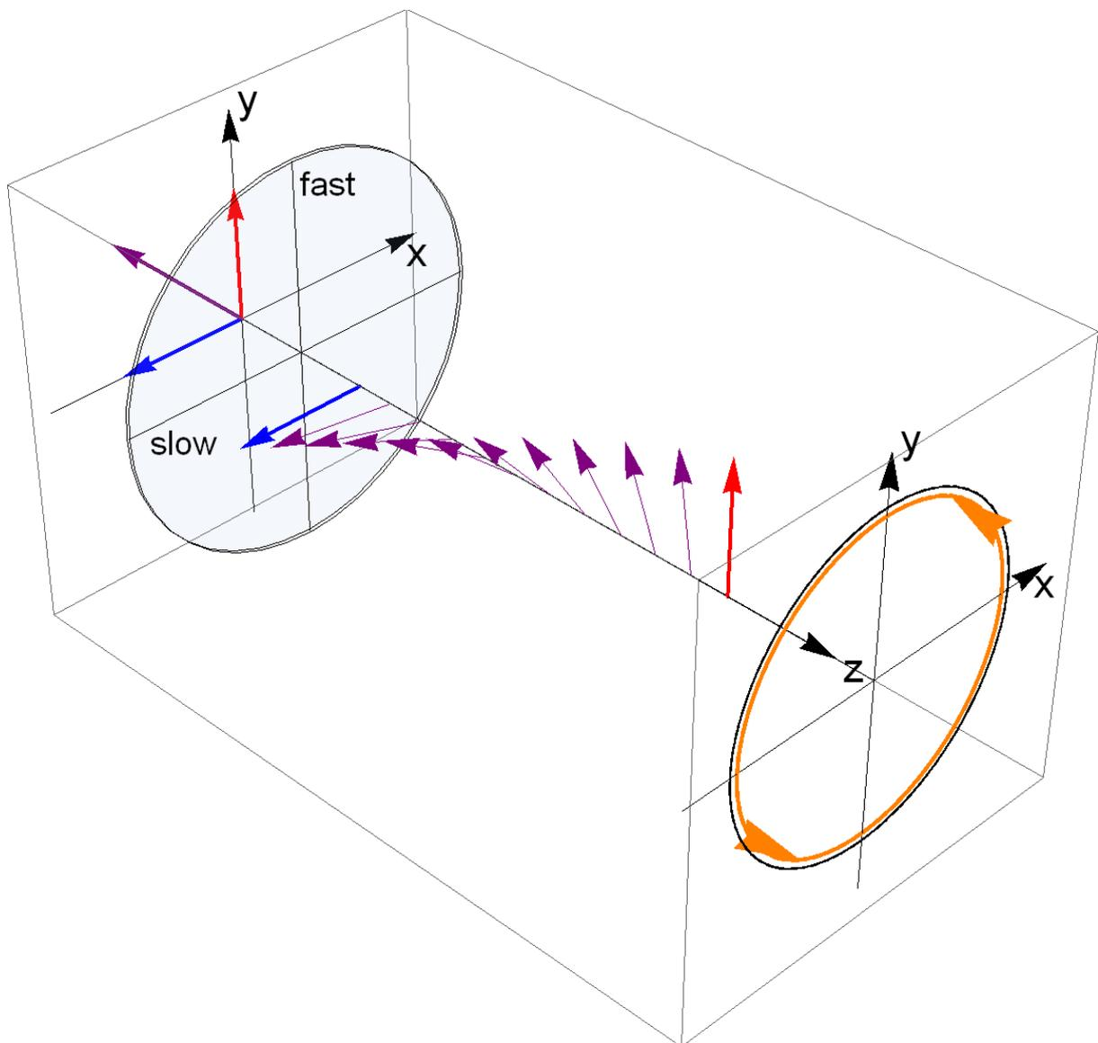
**Figure 4** The input polarization is  $-45^\circ$  linear and a left - hand circular polarization state is generated. The slow axis of the quarter waveplate is oriented along the x – axis.
