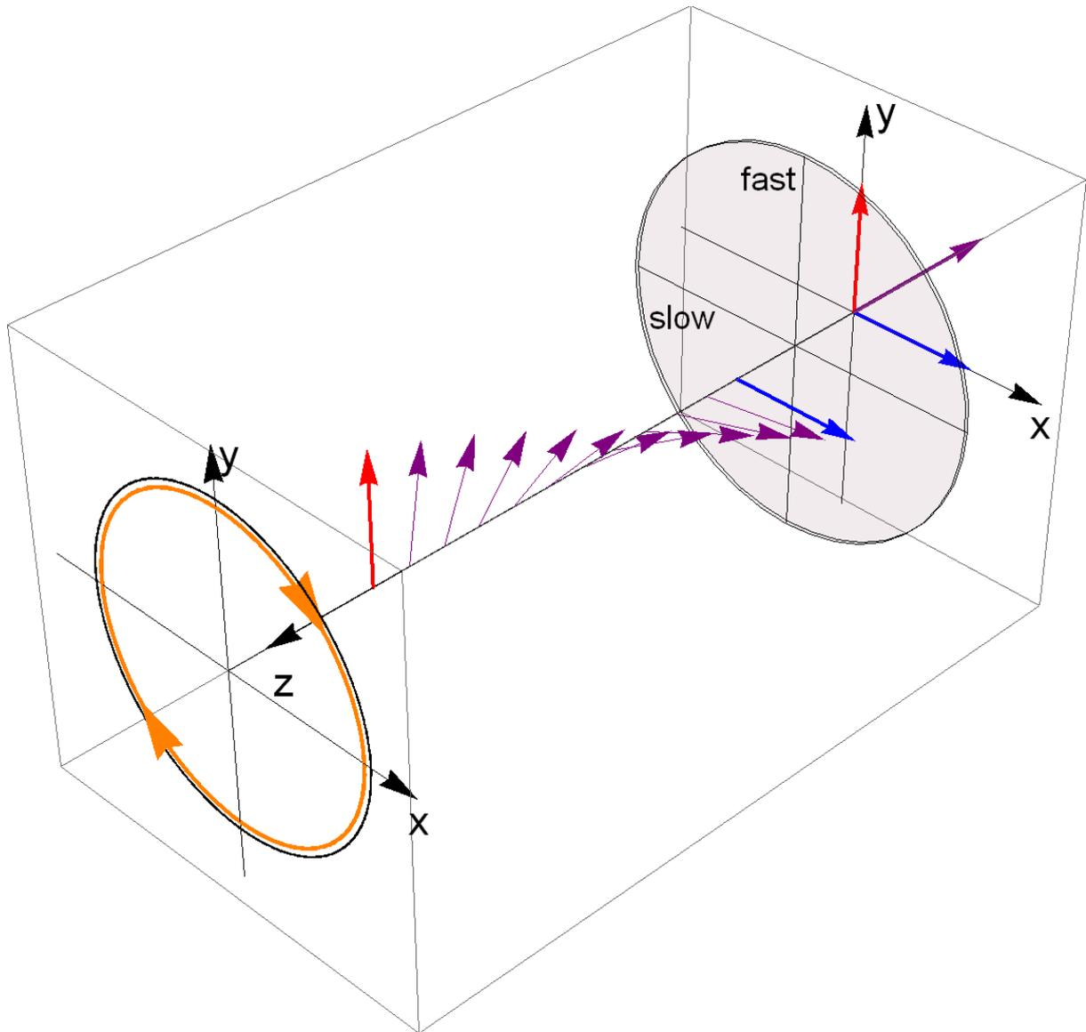
**Figure 3** The input polarization is +45° linear and a right - hand circular polarization state is generated. The slow axis of the quarter waveplate is oriented along the x – axis.
