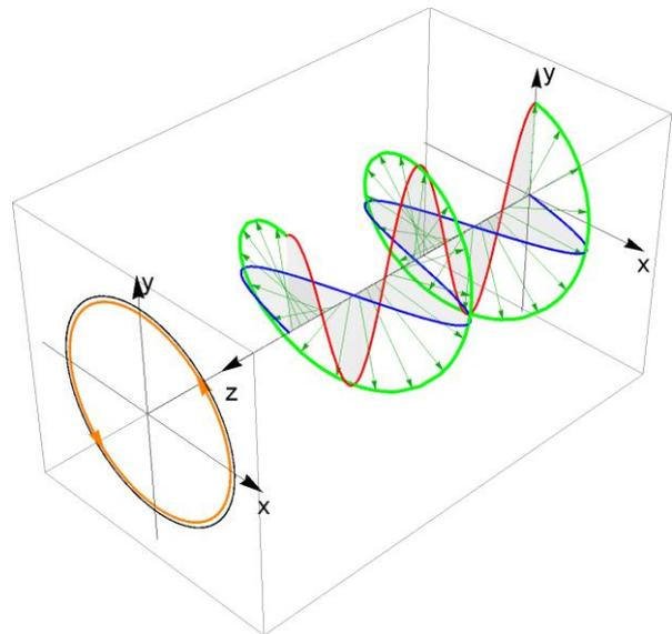
Figure 2 Left-Circularly Polarized Light
