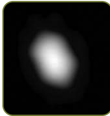
Measured Near Field Profile (log scale) of PM-1550-01
