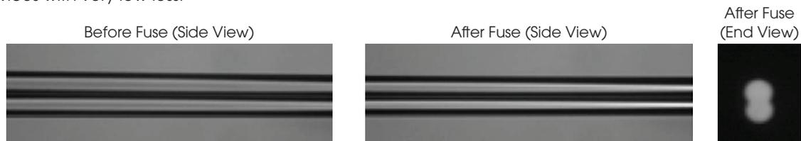
View from the glass processor of two single mode fibers tapered and fused together for 50:50 coupling. Spacing between the fiber cores is approximately 15 to 20 µm.
