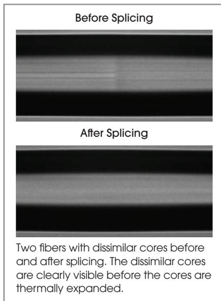
Two fibers with dissimilar cores before and after splicing. The dissimilar cores are clearly visible before the cores are thermally expanded.
