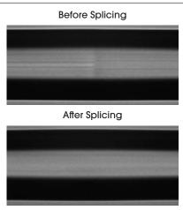
Two fibers with dissimilar cores before and after splicing. The dissimilar cores are clearly visible before the cores are thermally expanded.
