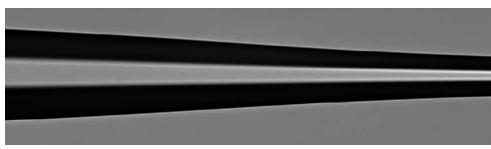
Ø20  $\mu m$  Core, Ø400  $\mu m$  Cladding Large-Mode-Area (LMA) Fiber Tapered to Ø125  $\mu m$  Cladding
