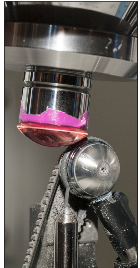
Diamond-Embedded Ferrofluids Polishing an Asphere in an MRF Polisher
