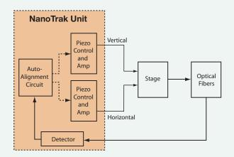
With one fiber fixed and the other mounted on a piezo-actuated stage capable of moving the fiber perpendicular to its endface, the NanoTrak<sup>TM</sup> controls the position of the moving fiber. The NanoTrak's auto-alignment circuit controls the fiber's position as it optimizes the coupling efficiency through the two fibers. In many applications, a planar waveguide or other device replaces one of the fibers; however, the basic principles remain the same.
