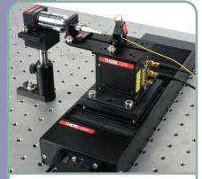
The fiber launch application photo above shows an APB301 PiezoBlock<sup>TM</sup> mounted on an NR150 150 mm travel stage (using an APBP2 adapter plate). The top plate of the PiezoBlock<sup>TM</sup> can be replaced with one of our platform extension plates (AMA005 shown, see page 497). This extended mounting surface is convenient for attaching extra components and allows easier access into smaller spaces.
