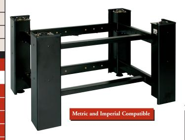
This family of passive isolation systems incorporates four independent air mounts for general applications requiring isolation from low frequency vibrations. Each leg is manually controlled to achieve a level surface and does not require a constant source of air to maintain the setting.
