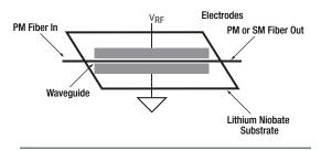
Phase Modulator Waveguide
