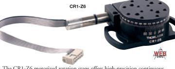
The CR1-Z6 motorized rotation stage offers high-precision continuous motion in a sturdy, compact package. The backlash-free worm gear design coupled with a high-resolution optical encoder provides the rotational precision required in optical laboratories. The high torque 12V DC Servo Motor supplies ample power for rotating vertical loads as high as 25 lbs.
