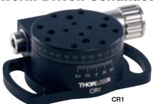
The CR1 rotation stage provides high precision along with low backlash. The low backlash is achieved with an anti backlash gear in the worm gear mechanism. The added ability to stack our line of translation stages on the rotation platform makes this stage useful in any lab.
