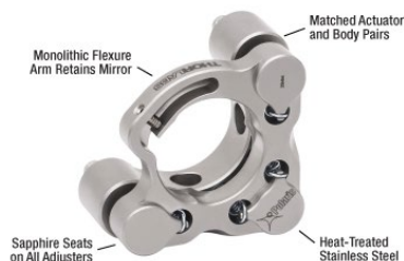
Click to Enlarge Details of the POLARIS-K1S4 Design. Note that some mounts on this page use a flexure spring to retain the optic and have bronze bushings instead of matched actuator/body pairs.
