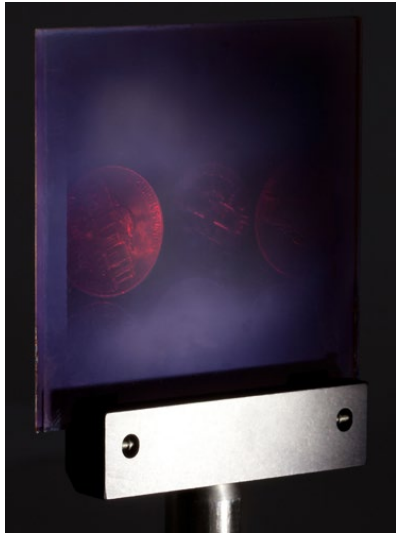
Figure 2: A reflection hologram viewed by reflecting light off of the plate.
