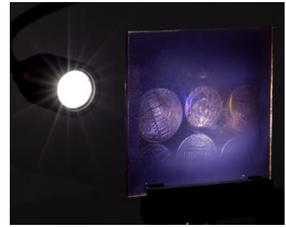
Figure 3: A reflection hologram viewed by transmitting light through the plate.
