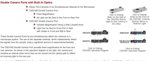
In contrast, the CSD1001 Double Camera Port offers fixed magnification for the front camera and variable magnification of 0.35X, 2X, or 4X for the rear camera.
