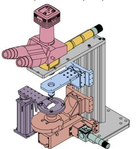
Breadboard: A flat structure with regularly spaced tapped holes for DIY construction.
