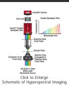
Click to Enlarge A hyperspectral imaging system built using Thorlabs' Cerna Microscopy Platform, KURIOS-VB1 Tunable Bandpass Filter, and Monochrome Scientific Camera. Several components shown here were modified from their stock configuration.
