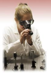
Viewing an IR Laser Beam with an IR Viewer
