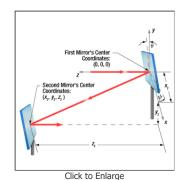
**Figure 3**: The beam reflected from Mirror 1 will be incident on Mirror 2, if Mirror 1 is rotated around the *x*- and *y*-axes by angles  $\theta$  and  $\psi$ , respectively. Both angles affect each coordinate ( $x_2$ ,  $y_2$ ,  $z_2$ ) of Mirror 2's center. Mirror 1's rotation around the *x*-axis is limited by the travel range of the mount's pitch (tip) adjuster, which limits Mirror 2's position and height options.
