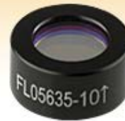
FL05635-10 Ø1/2" Filter CWL = 635 nm, FWHM = 10 nm
