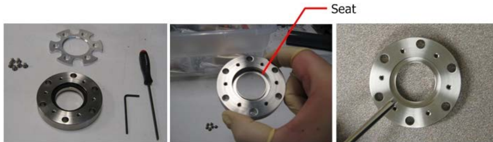
Left: Viewport with front face removed. Middle: O-Ring is removed, inspect the seat. Right: Using compressed air, remove loose debris from the seat.
