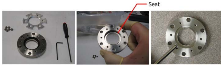
Left: Viewport with front face removed. Middle: O-Ring is removed, inspect the seat. Right: Using compressed air, remove loose debris from the seat.
