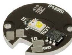
M565D2 565 nm LED, Power Output > 880 mW
