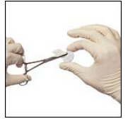
Click to Enlarge Optic Cleaning Using Forceps and Lens Tissue Paper
