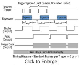
**Figure 1:** Streaming overlapped exposure mode. When the external trigger goes low, the exposure begins, and continues for the software-selected exposure time, followed by the readout. This sequence then repeats at the set time interval. Subsequent external triggers are ignored until the camera operation is halted.
