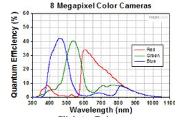
This curve shows the quantum efficiency for the color camera sensor's red, green, and blue pixels.
