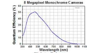
This curve shows the quantum efficiency for the monochrome camera sensor.
