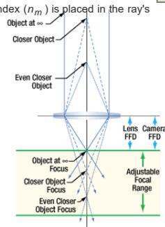
**Figure 10:** When their flange focal distances (FFD) are the same, the camera's sensor plane and the lens' focal plane are perfectly aligned. Images of objects at infinity coincide with one limit of the system's focal range.
