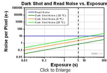
**Figure 1:** Plot of dark shot noise and read noise as a function of exposure for three sensor temperatures for our 1.4 megapixel cameras. This plot uses logarithmic scales for both axes. The dotted vertical line at 5 s indicates the values calculated as the example in the text.
