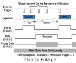
**Figure 2:** Asynchronous triggered acquisition mode. When the external trigger signal goes low, an exposure begins for the preset time, and then the exposure is read out of the camera. During this readout time, the external trigger is ignored. After a single readout is complete, the camera will begin the next exposure only when the external trigger signal goes low.
