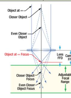
**Figure 11:** Tolerance and / or temperature effects may result in the lens and camera having different FFDs. If the FFD of the lens is shorter, images of objects at infinity will be excluded from the focal range. Since the system cannot focus on them, they will be blurry.
