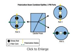
then the light will be deviated by the prism such that it emerges from port 2 with the light aligned to the slow axis. Note that the slow axes of the fibers on port 1 and port 2 are orthogonal to each other to match the polarization emitted by the calcite prism. If the polarization incident on port 3 is at an angle with respect to the axes, the output at ports 1 and 2 will vary depending on the angle of the incident polarization state.
