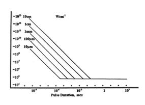
LIDT in linear power density vs. pulse length and spot size. For long pulses to CW, linear power density becomes a constant with spot size. This graph was obtained from [1].
