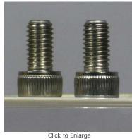
Figure 4: An image of two identical 8-32 cap screws imaged with our MVTC23013 0.128X Telecentric Lens. Although the screws appear to be the same size and in the same object plane, they are actually separated by a distance of approximately 45 mm along the optical axis.
