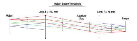
Figure 1: A ray trace through an idealized object space telecentric lens system. Note that the chief rays (the center ray of each color) is parallel to the optical axis in object space, but in image space, the chief rays form an angle with the optical axis.
