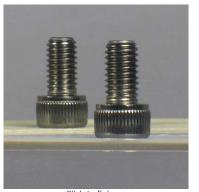
Click to Enlarge Figure 5: The same two screws photographed with our MVL7000 conventional zoom lens. In this image, the perspective error due to the separation of the screws would lead to incorrect height measurements.
