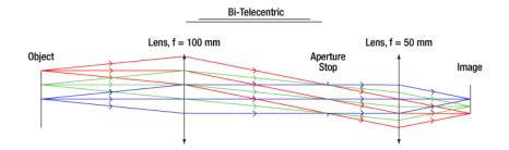
Figure 2: A ray trace through an idealized bi-telecentric lens system. Note that the chief rays (the center ray of each color) is parallel to the optical axis in both image and object space, which means that the magnification will remain constant regardless of object distance.
