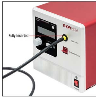
Figure 2: As shown above, the LLG is correctly installed when the edge of the yellow band is flush with the front panel of the light source.
