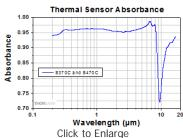
This absorption curve is shown over a broader wavelength range than the sensors' operating ranges. See the table for the operating wavelength range of each sensor.
