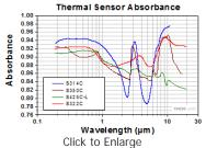
The absorption curves of each of the thermal power sensors designed for use with low and medium power optical sources.
