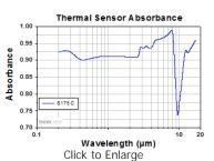
Typical absorption curve for the S175C (glass and absorber). Note that this curve is representative, and the actual absorption across the spectrum will vary from unit to unit.
