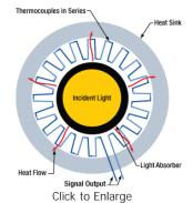
Figure 1: A thermal sensor with radially configured thermocouples, which is depicted as seen from the top. Light is incident on the absorbing layer at the center, and heat flows through the thermocouples to the heat sink.
