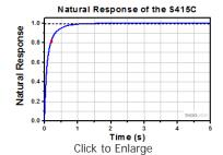
Figure 3: Natural response of the S415C with the dotted line at 99% and the red square indicating the point on the curve corresponding to a single sensor time constant.
