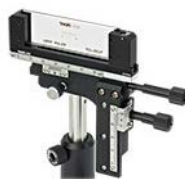
Click to Enlarge An R1L3S1P Stage Micrometer Mounted in an XYFM1 Test Target Positioner
