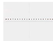
Click to Enlarge Close Up of the R1L1S5P Horizontal Scale with Crosshair
