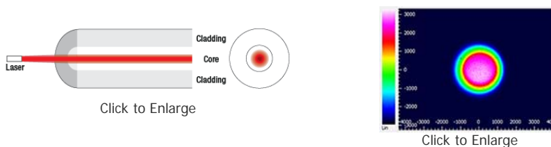
Diagram illustrating an underfilled launch condition (left) and a beam profile measurement using a FT200EMT multimode fiber (right).
