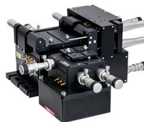
Click to Enlarge In the Above Application, a 3-Axis NanoMax Flexure Stage is Aligned in Front of a 6-Axis Stage at the Proper 112.5 mm Deck Height Using an AMA554 Height Adapter
