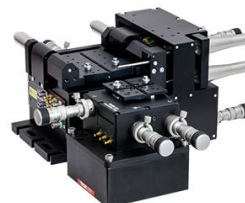
Click to Enlarge In the above application, a 3-Axis NanoMax flexure stage is aligned in front of a 6-axis stage at the proper 112.5 mm deck height using an AMA554 Height Adapter.
