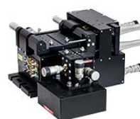
Click to Enlarge Figure 7: In the Above Application, a 3-Axis MicroBlock Compact Flexure Stage is Aligned in Front of a 6-Axis Stage at the Proper 112.5 mm Deck Height Using an AMA554 Height Adapter
