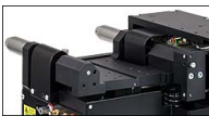
Figure 4: The stainless steel probe can be removed at any time by loosening the knurled knob on the front of the stage.
