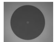
Click to Enlarge Undamaged Fiber End
