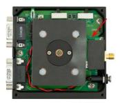
Figure 3. TCLDM9 Internal Circuitry Showing Jumper J4 Click to Enlarge
