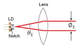
Figure 2. Parallel beam divergence from L785P025 style A laser diode
