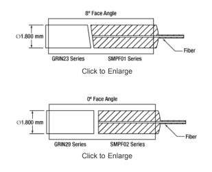
All GRIN Lens / Pigtailed Ferrule combinations require a 51-2800-1800 mating sleeve, shown below. To build the device, insert the lens and ferrule into opposing sides of the sleeve, gently bring them into contact to ensure that the faces are parallel, then bring the lens and ferrule apart until the desired focusing is achieved.
