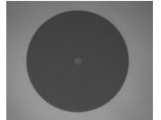
Click to Enlarge Undamaged Fiber End
