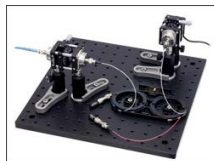
Click to Enlarge Setup to Measure Extinction Ratio of a 1550 nm PM Coupler
