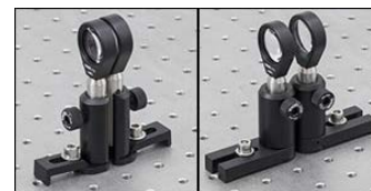
Click to Enlarge Close-Approach Post Holders can Mount Ø1/2" Posts in Contact, while Posts Mounted in Standard Post Holders are Separated by a Minimum of 0.48" (12.2 mm)
