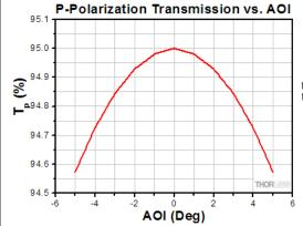
Click to Enlarge Percent transmission of ppolarized throughput beam. AOI is measured from the normal of the polarizer's face plate.
