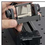
Click to Enlarge Prism Mirror Mount is Easily Installed and Removed using Three 8-32 (M4) Cap Screws
