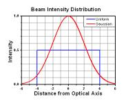
hotspots in the beam or other non-uniform intensity profiles and roughly calculate a maximum power density. For reference, a Gaussian beam typically has a maximum power density that is twice that of the uniform beam (see lower right).
