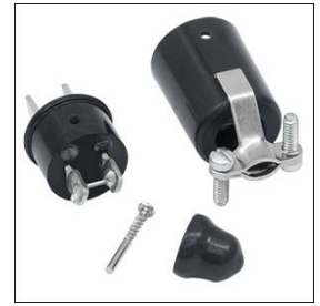
Click to Enlarge Third, remove the protective cap to expose the short wire, which can be desoldered.
