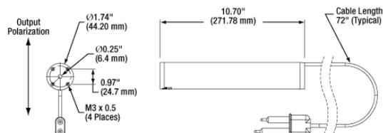
Thorlabs' cylindrical, 2.0 mW, red (632.8 nm) Helium-Neon lasers feature a tube design that makes them easy to mount in nearly any optical system. These lasers are offered with either linear (500:1 polarization ratio) or random polarization. The linearly polarized beam is polarized vertically with respect to the cable at the rear of the laser's housing. A built-in interlock circuit is included that can be integrated with lab safety systems (see *Interlock Disassembly* tab for details). The
