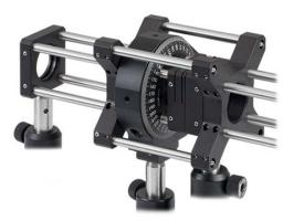
The PRM1Z8 can be aligned within a 30 mm cage system by using two LCP02 30 mm to 60 mm cage plate adapters, a CPR1 rotating cage segment plate, and three ER3 Cage Rods. This creates a motorized rotation mount within a rigid optical assembly. For more details on how the PRM1Z8 and CPR1 work together, please see the animation to the right.
